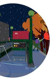
Low curb heights near subway entrances can't hold back stormwater from flowing over streets and sidewalks and down subway street stairways, to the mezzanine.
