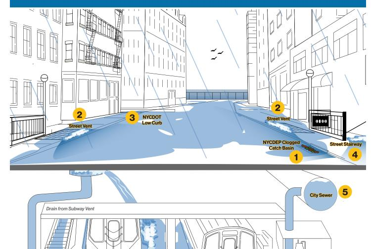
When large volumes of stormwater enter through vents and down street stairs, and when **city sewers (5)** are full and backup into stations, the underground drainage system becomes taxed. Stormwater can build up in mezzanines and on stairways and platforms, impacting customer experience. Subway service delays occur when stormwater floods tunnels and tracks (6). Subway service is shut down until the water is removed.
