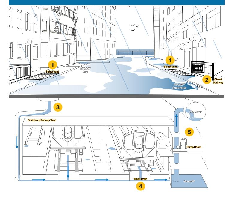
This system includes drain lines, **vent drains (3)**, **track drains (4)**, sump pits, and **pump rooms (5)**. It removes stormwater that enters by discharging to the city's sewer system. Stormwater then travels to a nearby wastewater resource recovery facility.
