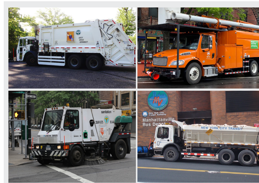
Examples of specialized government vehicles designed to perform specific public works include garbage collection trucks (top left); tree pruning trucks (top right); street sweepers (bottom left); and snow-removal trucks (bottom right).
