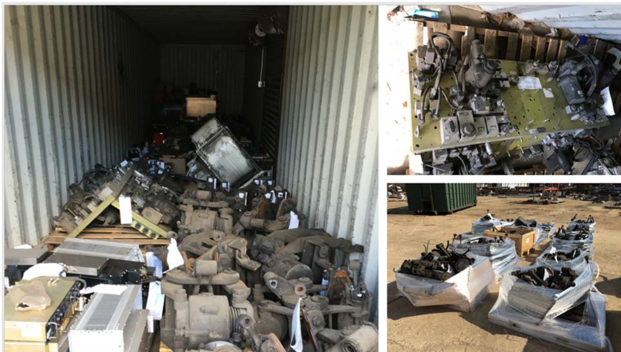
Figure 7. Brake System Components from Legacy Acela Trainset
