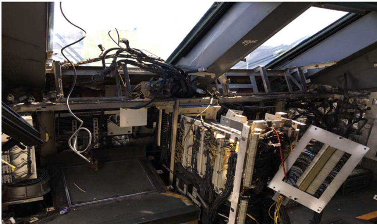
Figure 6. Legacy Acela Trainset Used for Spare Parts
