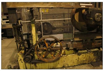
Figure 24. Rolling Load Machine at the TTC
