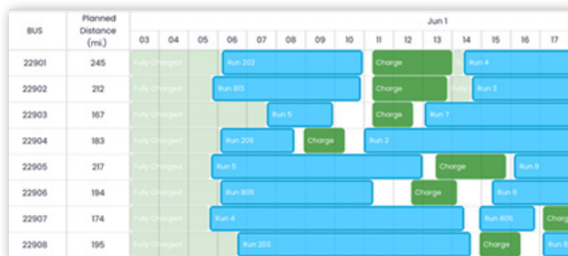
Widesense dashboard shows a new proposed charging schedule, with potential to increase utilization rates, for eight NJT buses at the Camden Garage.
