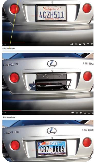
Figure 30 Legitimate license plate rotates... to display fake plate
