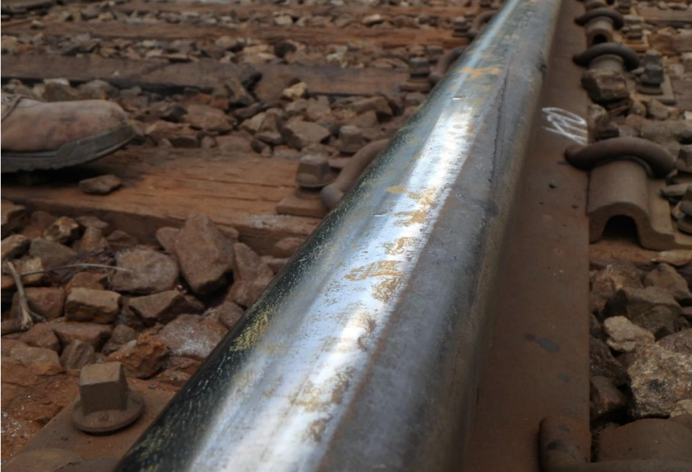
Figure 3. Photograph showing a section of rail with wheel flange departure mark across the rail in curve at the Point of Derailment.
